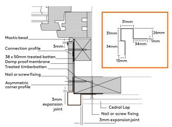
Use on right and left vertical of windows and doors allowing for lapped boards on face side of building and single board laid flat around the reveal of window or door.
