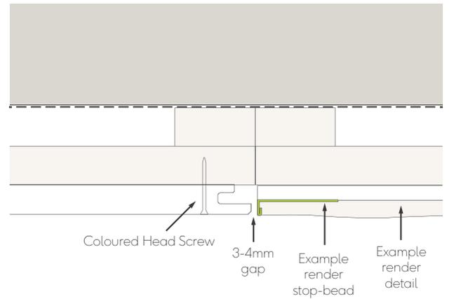
Fig. 21 - Corner profile butting up to render
