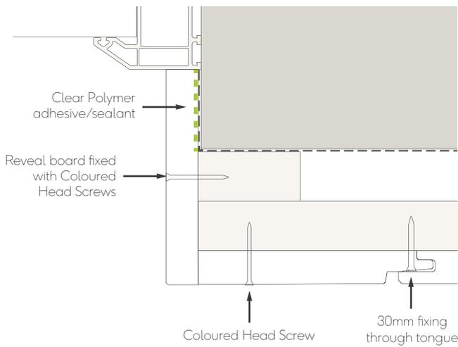
Fig. 11 - Window/door jamb with Reveal board
