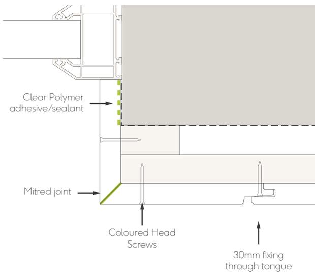
Fig. 13 - Window/door jamb with mitred joint
