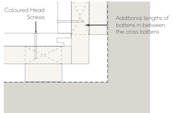
Fig. 9 - Internal butt joint corner detail
