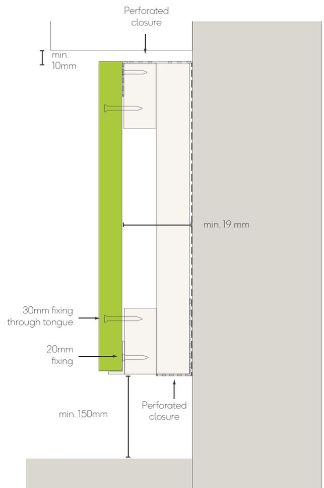
Fig.1 - Top & bottom of cladding detail
