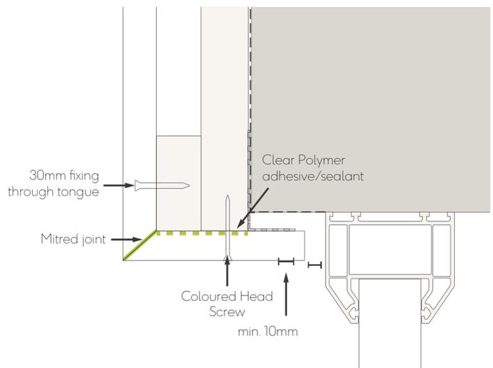
Fig. 14 - Window/door head with mitred joint
