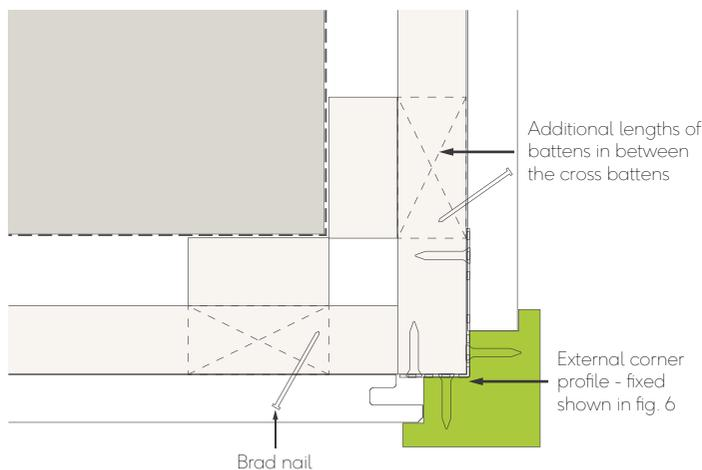
Fig. 16 - External corner detail - brad nails
