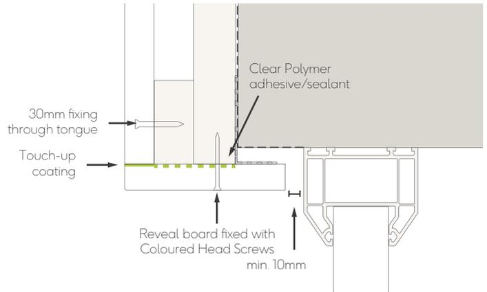
Fig. 12 - Window/door head with Reveal board
