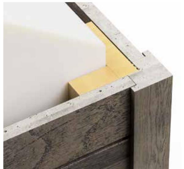
Alternatively, the boards can be butted together on an internal corner as shown in fig. 9. The boards can also be mitred to create the external corner, this would also be applicable if the corner is anything other than 90 degrees.
