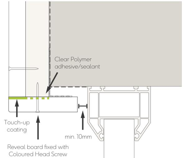
Fig. 12 - Window/door head with Reveal board
