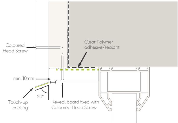
Fig. 15 - Window/door head with angled cut
