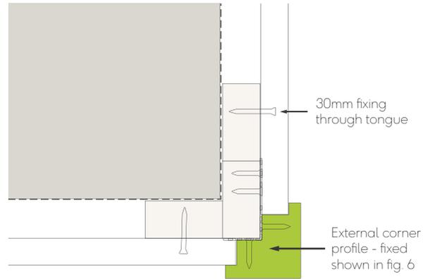
Fig. 8 - External corner detail
