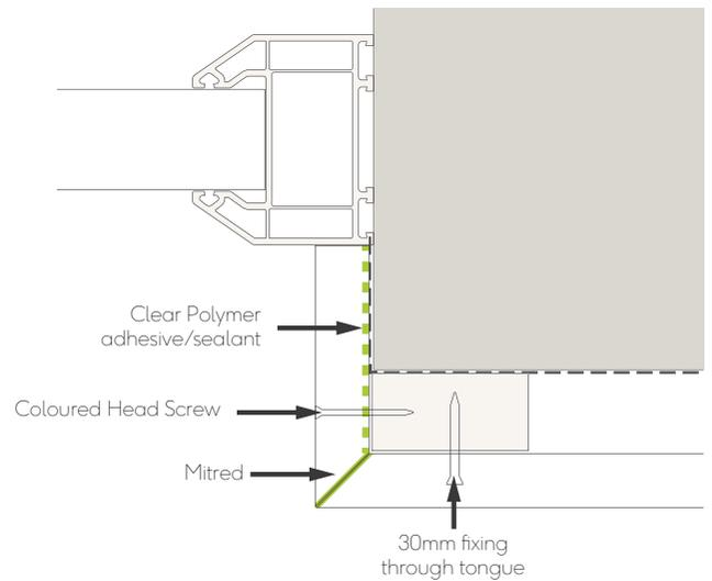
Fig. 13 - Window/door jamb with mitred joint
