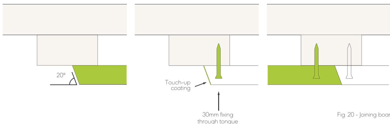
Fig. 20 - Joining boards detail
